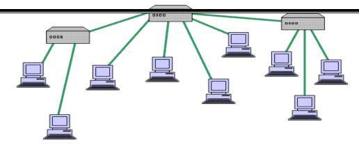
These condary hub maybe active or passive. A passive hub means it just precedes a physical connection only.
